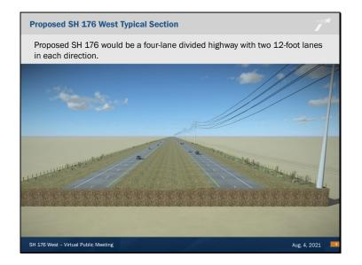
The proposed typical section for SH 176 would be a four-lane divided highway with two 12-foot lanes in each direction.
