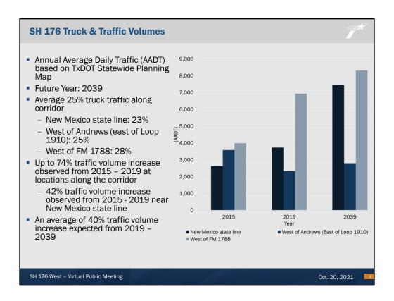
Traffic volumes on SH 176 were analyzed using the TxDOT Statewide Planning Map and using years 2015, 2019, and 2039 for comparison. Up to a 74% increase in traffic volume was observed from 2015 to 2019 at locations along the corridor. A 42% increase in traffic volume was observed near the New Mexico state line.
