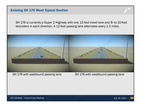
Within the project limits, SH 176 is currently a Super 2 Highway with one 12-foot travel lane and 8 to 10-foot shoulders in each direction. A 12-foot passing lane alternates every 1.2 miles.
