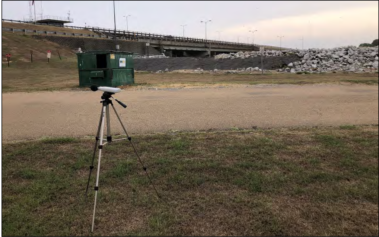
Near boat launch parking lot, aiming northeast (NM02). An earthen berm pictured above shielded the measurement from noise pollution caused by water flow from dam.
