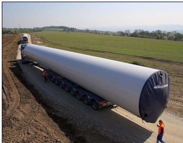
Figure 13: Transporting a Wind Turbine Tower Component
