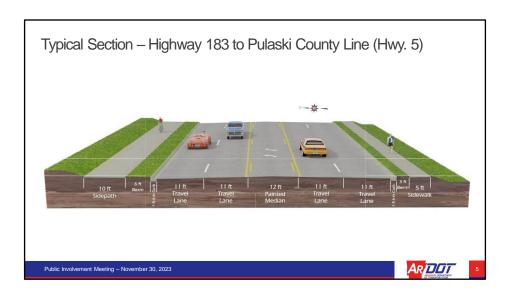
The typical section for the proposed widening of Highway 5 consists of four 11-foot-wide travel lanes, and one 12-foot-wide painted median.
