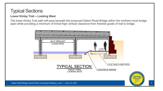
Maintaining a westward view, the lower Kinley Trail path will pass beneath the proposed Salem Road Bridge within the northern most bridge span while providing a minimum of 9-foot-high vertical clearance from finished grade of trail to bridge.
