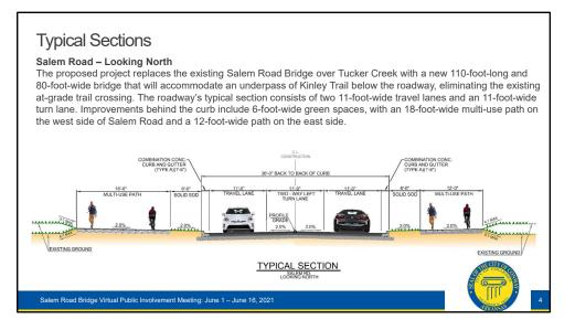
The proposed project replaces the existing Salem Road Bridge over Tucker Creek with a new 110-foot-long and 80-footwide bridge that will accommodate an underpass of Kinley Trail below the roadway, eliminating the existing at-grade trail crossing.
