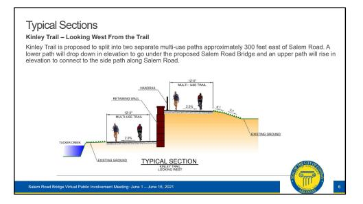
When looking west from Kinley Trail, the trail is proposed to split into two separate multi-use paths approximately 300 feet east of Salem Road. A lower path will drop down in elevation to go under the proposed Salem Road Bridge and an upper path will rise in elevation to connect to the multi-use path along Salem Road.
